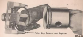
Fig. 24—Installing Piston Ring on Piston
