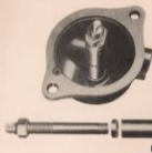
Fig. 40—Removing Governor Bushing
