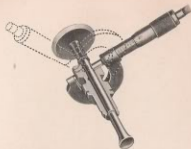
Fig. 29—Checking Valve Guide Bushing for Wear
