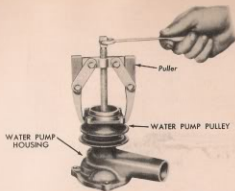
Fig. 33—Removing Water Pump Pulley
