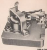
Fig. 43—"Go" and "No Go" Gauge Inserted Behind Governor Lever
