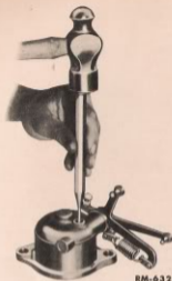
Fig. 38—Driving Grooved Pin from Fork and Lever
