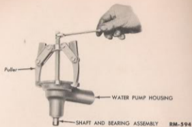
Fig. 35—Pressing Bearing and Shaft from Pulley Hub
